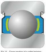
Fig. 5: Cross-section of a roller bearing filled with Turmocomp HD 150
